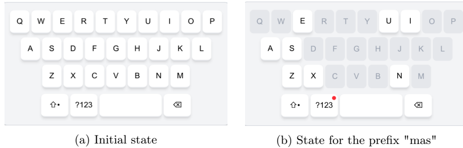
Fig. 2: Prototype virtual keyboard showing the initial state and a blocked-key state for prefix “mas”
